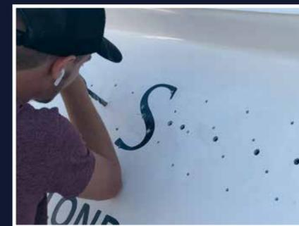
Together with each lettering we deliver an exact template with the precise positions of the drill holes for the bolts and the electricity supply.
