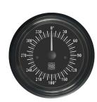
Professional instrument for measuring the angular position on 0-360° in the dimension Ø100mm. Available with 0,5-4,5V input and 12/24V power supply.
