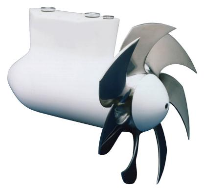
Available in five sizes and seven power levels for bow and stern applications, the NAIAD® In-Line Hydraulic Thruster is an extraordinarily compact unit with high output relative to its tunnel diameter. A unique feature of this design is the highly skewed propeller offering maximum thrust and extremely quiet operation. The thruster housing, propeller and shafting are precision manufactured in AISI 316 stainless steel for superior marine corrosion resistance.
