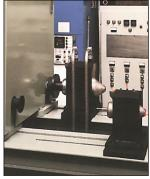
Unlike other thrusters which, if tested at all, are simply cycled, our thrusters are rigorously tested under full load on our unique Dynamometer Test Stand. They are cycled in continuously reversing rotation against a propeller shaft load to dynamically test the performance of the bearings, seals and hydraulic motor.
