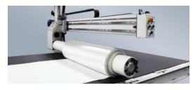
Manage long cut pieces with ease and minimize labor by streamlining your material handling operations after cutting. Eastman rewinder nodes work in synchronization with the conveyor cutting system to roll up cut pieces onto a core as they convey off of the cutter. Waste material continues to move along the system or drop into a collection bin. The rewinders are particularly useful when cut parts exceed the table length and become difficult for operators to collect manually.
