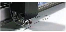
Eastman's various JetPRO inkjet systems are Drop-on-Demand (DOD) printers which convert TEXT entities from a drawing file and prints them directly with the printing head mounted on the cutting gantry. The result is very fast throughput compared to traditional pen or airbrush.
