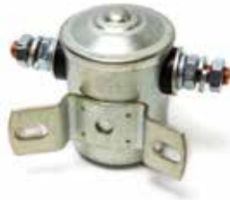
18-5840 SOLENOID Replaces: Prestolite 15-79, SAW4201, SAW4207, SAW4210 Steel housing copper contacts * 12 Volts grounded Continuous rating: 85 amp @ 12 VDC
