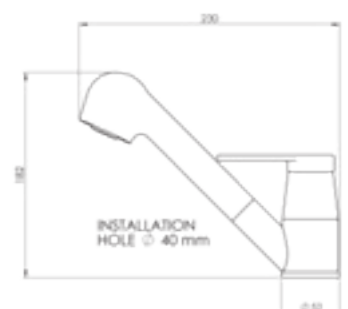
Single control tap with removable shower mounted on 1500 mm flexible tube Hot and cold water.
