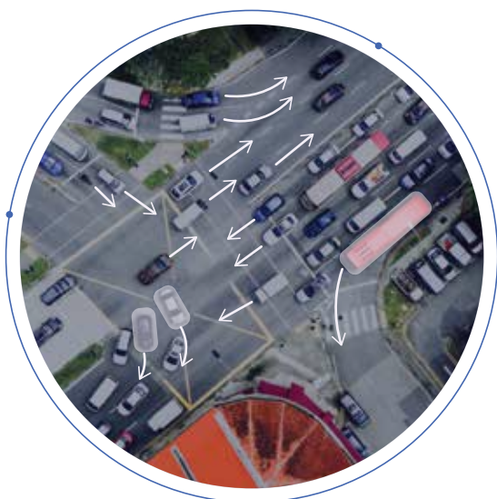
Intersection monitoring with origin – destination detection and left-turn compliance monitoring
