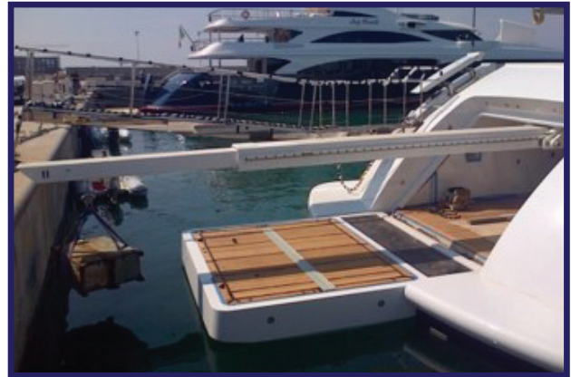
Overhead telescopic crane
