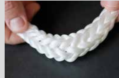
Single braid Dyneema® without HPS treatment: the braid is soft and "airy".
