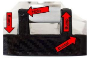
**Surface:** irregular, created by adding fabrics and resin over a grossly shaped foam core.
