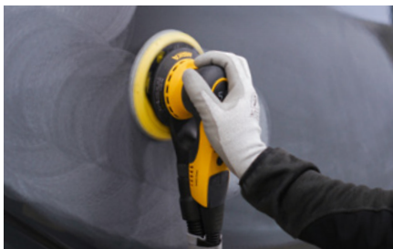
Mirka® DEROS 650CV 150 mm, orbit 5 mm
