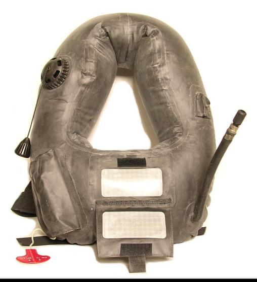
SOS Marine`s UDT lifejacket is a universal device of compact and durable design. The purpose is to provide emergency flotation for Naval Clearance divers and other divers conducting military operations
